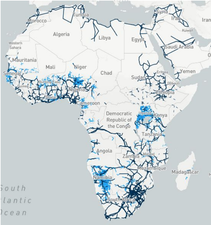
Figure 2: Africa's Existing and Planned Low, Medium, and High Voltage Transmission Lines 18
